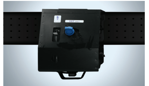
Frame-mounted DEF tank is easy to reach and fill, and comes covered with heating system
