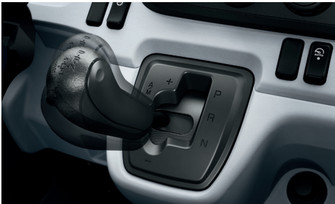
Dash-mounted shifter provides easy cross-cab access
