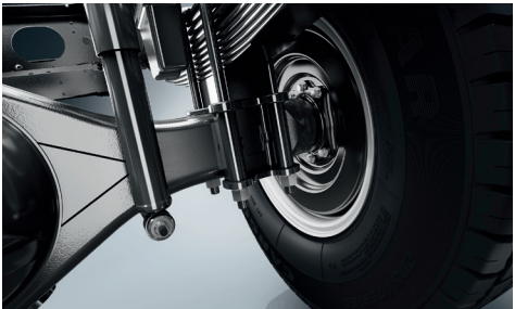
Rugged rear shock absorbers and multi-leaf suspension
