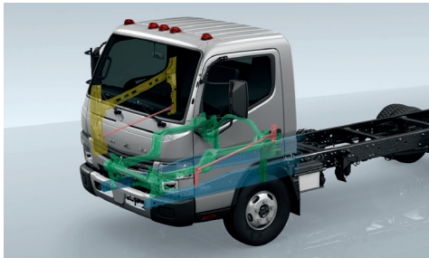
Long-term anti-corrosion treatment applied in factory
